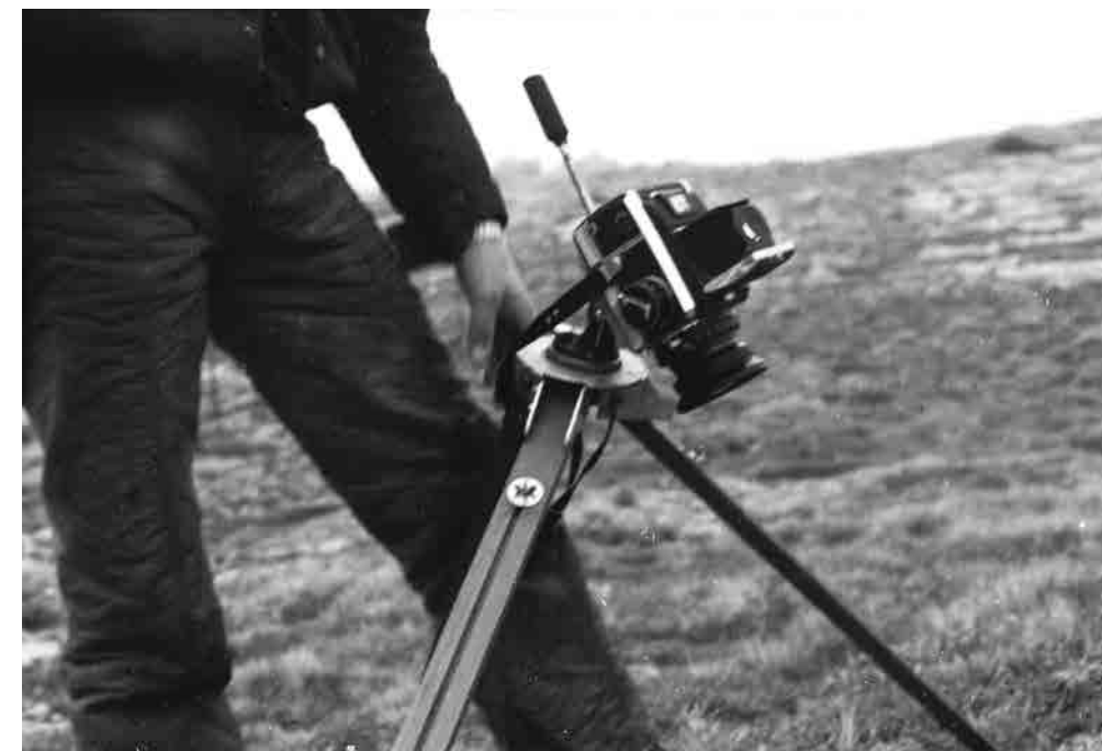
The series was shot with a 40 mm lens on a 6 x 6 cm format camera which offered a wide angle of view and good depth of field.
