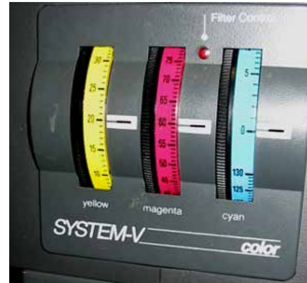
Filter dials on a colour enlarger yellow magenta cyan. Traditional photography might use increments to 25 cc - for the photograms increments up to 130
